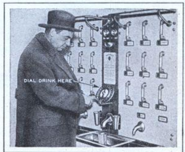
Dialing number of soft drink or wine delivers a shot from the spigot, thus eliminating customary bar tenders.
